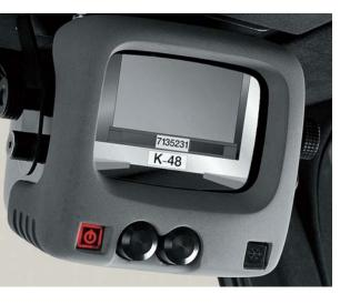
**Lift height preselector** is programmable for up to 99 shelf levels for safe, precise and economical load handling at any height.
