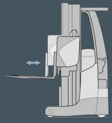
The fork carriage traverses backwards and forwards and has a very short travel distance.
